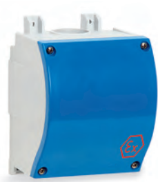
ULYSSE-Ex SERIES ATEX enclosures with blind cover, in thermosetting (GRP) material with double protection rating IP66 / IP67
