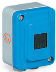
TAIS-MIGNON-Ex SERIES ATEX push-button in watertight wall-mounting enclosure in thermosetting (GRP) material IP66 / IP67
