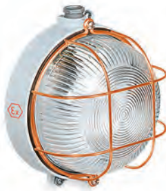
RINO-Ex SERIES ATEX grey watertight round lighting fixture in aluminium alloy RAL 7035, tropicalized steel wire protective cage and glass diffuser 250V - IP65
