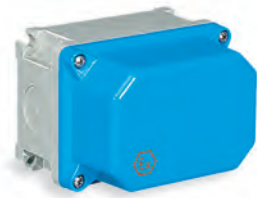
TAIS-Ex SERIES ATEX watertight enclosures with raised cover in thermosetting (GRP) material IP66 / IP67
