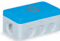
TAIS-MIGNON-EX SERIES ATEX watertight wall-mounting modular coupling box in thermosetting (GRP) material IP66 / IP67
