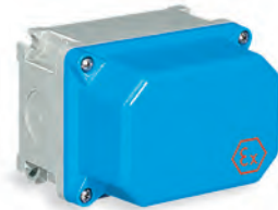
TAIS-Ex SERIES Watertight wall-mounting blind enclosures with ATEX high cover, in thermosetting (GRP) material IP66 / IP67
