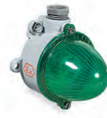
RONDÒ-EX SERIES ATEX wall-mounted signal lamps in watertight aluminium alloy enclosure IP54
