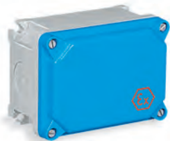
TAIS-Ex SERIES Watertight wall-mounting blind enclosures with ATEX low cover, in thermosetting (GRP) material IP66 / IP67
